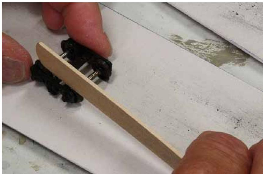
Turn the wood over for the opposite wheel. Note the dirt picked up from the wheel that was just polished. Swap the tongue depressor end for end for the other axle so that each wheel gets polished with a clean edge. Use the sandpaper to clean up the tongue depressor for the next set of wheels. There may be some “lint” on the treads after polishing. I use an old toothbrush to remove that.
