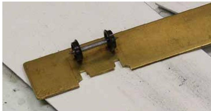
If the wheels are in gauge and centered, they will fit right in. If not, a quick visual inspection shows where an adjustment is needed. The slots for the wheels are just a smidge wider than the tread, so I can feel a very slight side to side motion if the spacing is correct. If I feel a bind, the wheels need adjusting.
