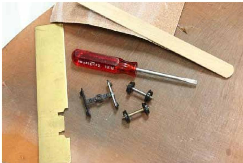
Here is a set of dirty wheels from my collection. I've noted that as the gunk builds up and gets thicker, it changes the geometry of the wheels; and they become prone to derailing, especially on turnouts. When a car derails, the first thing I check is for dirt on the treads.
