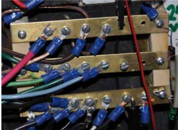
I had been using Radio Shack's "Solder Type Terminal Strips". They are relatively inexpensive and in some cases are perfect for connecting wires. But they require soldering. So I came up with the above "Bus Bar" to connect multiple wires to a power source. This uses 1/2" x 1/8" brass bar stock available from Ace Hardware. Each bar has several holes drilled and tapped for 4-40 screws spaced 3/8" apart. All my ground wiring is now connected together in one spot with solder-less crimp connectors.
